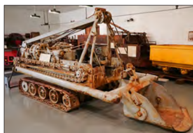
The Big Joe Shovel, essentially a mechanical loader on crawler tracks, was designed by the St. Joseph Lead Co. and engineered to the specific underground conditions in the Old Lead Belt. Only 52 were built, the first around 1922.
